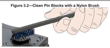
5. Inspect the Master and Tool pin blocks for stuck pins or severe pin block damage.
