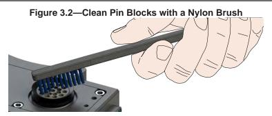
5. Inspect the Master and Tool pin blocks for stuck pins or severe pin block damage.
