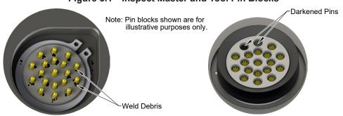
Tool Module Pin Block
