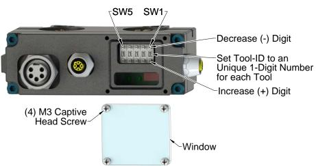
Figure 2.5—Tool-ID Switch Settings
