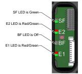
The System Failure (SF) status LED is identified on the module as "SF". It provides device status for power and proper operation. Refer to *Table 2.4* for an outline of this LED's operation.
