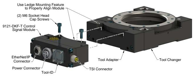
Figure 3.2—DKF-T Module Installation
