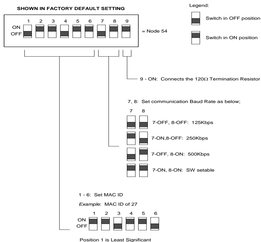
Figure 3.1—DeviceNet Master Module DIP Switch Settings
