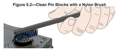
9. Inspect the Master and Tool pin blocks for stuck pins or severe pin block damage.
