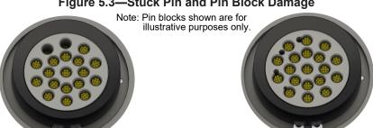
Figure 5.3—Stuck Pin and Pin Block Damage
