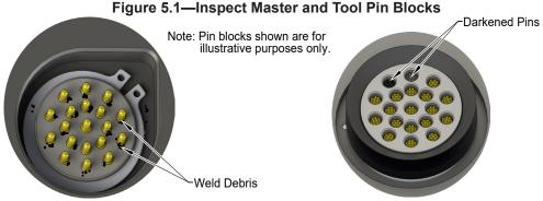
Tool Module Pin Block
