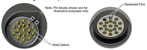
Tool Module Pin Block
