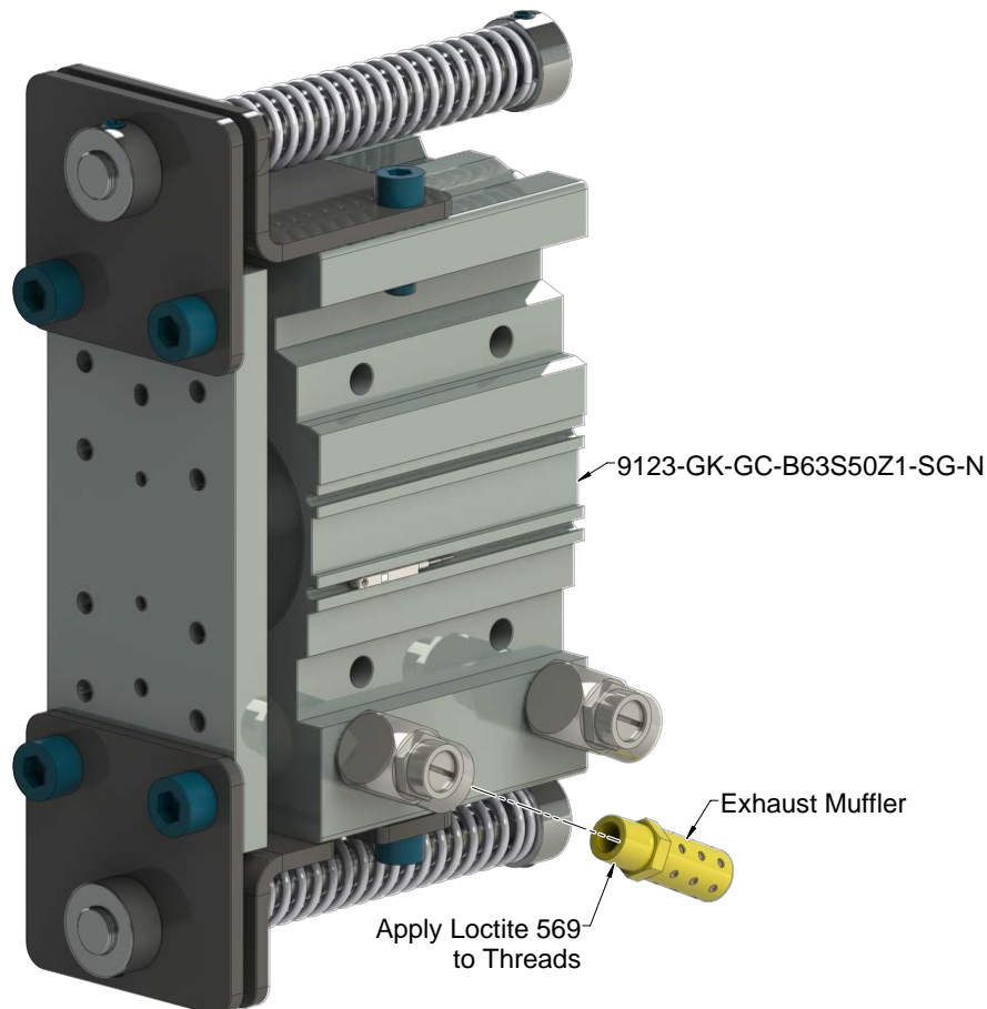
Figure 5.18—Exhaust Muffler Replacement
