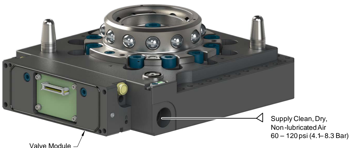
Figure 2.5— Master Side Pneumatic Connections
