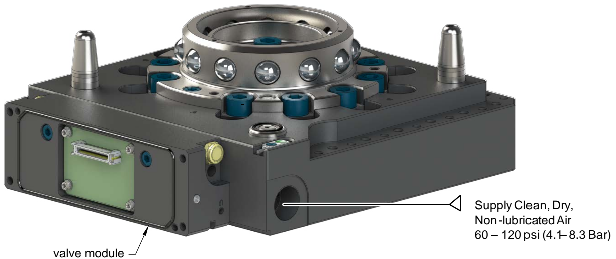
Figure 2.8—Pneumatic Connections
