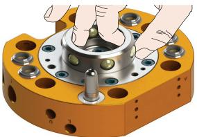
7. Apply a liberal coating of lubricant to the ball bearings, the male coupling (inside and out), and the alignment pins.
