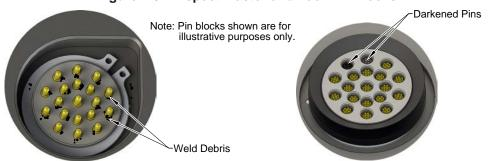
Tool Module Pin Block
