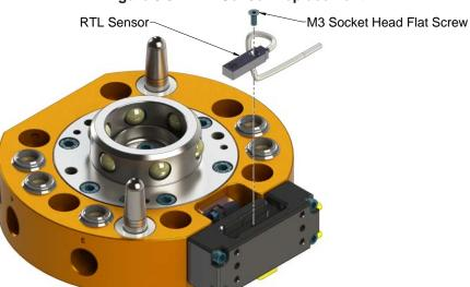
Figure 5.3—RTL Sensor Replacement
