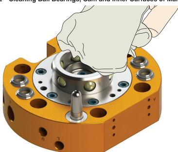
6. Check each ball bearing to make sure it moves freely in the male coupling. Additional cleaning may be necessary to free up any ball bearings that are sticking in place.
