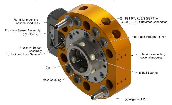
Figure 1.1—Master Plate Assembly (Shown with Optional Sensors)
