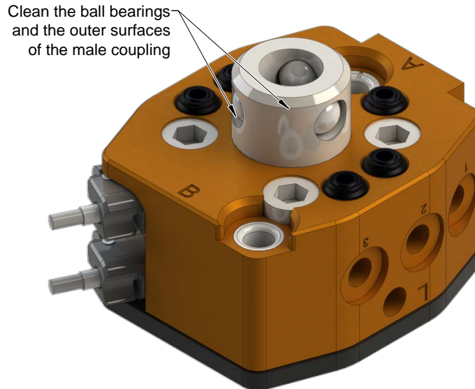
Figure 4.1—Cleaning Ball Bearings and Outer Surfaces of Male Coupling
