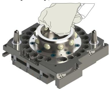
6. Check each ball bearing to make sure it moves freely in the male coupling. Additional cleaning may be necessary to free up any ball bearings that are sticking in place.
