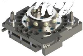
7. Apply a liberal coating of lubricant to the ball bearings, the male coupling (inside and out), and the alignment pins.
