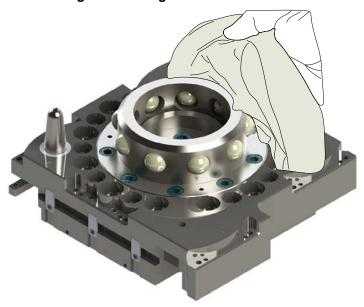
5. Use a clean rag to thoroughly remove any lubricant and debris from the inner surface of the male coupling and cam.
