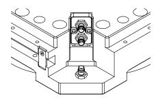
Lock and Unlock Sensor Assemblies
