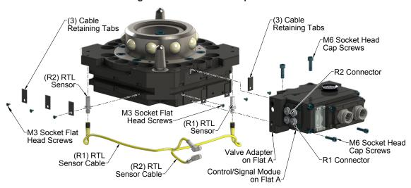
Figure 5.5—RTL Cable Replacement
