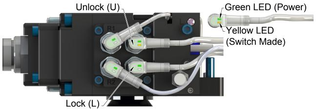
18. Confirm the operation of the Lock sensor by locking the Tool Changer and verifying the Lock sensor cable LED is on.
