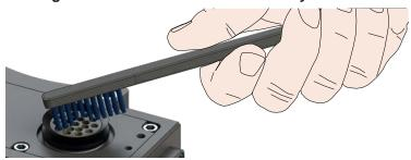
5. Inspect the Master and Tool pin blocks for stuck pins or severe pin block damage.
