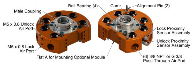
Tapered pins located on the Master plate mate with bushings in the Tool plate to ensure repeatable alignment during the coupling process. An extreme pressure grease is applied to the cam, male coupling, ball bearings, and pins to enhance performance and maximize the life of the Master plate assembly.
