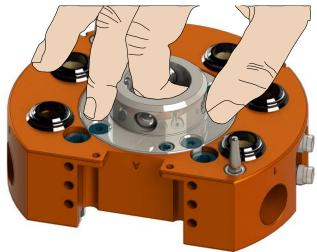
7. Apply a liberal coating of lubricant to the ball bearings, the male coupling (inside and out), and the alignment pins.
