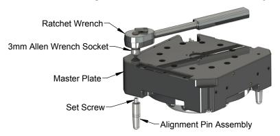
7. Once the alignment pin has been removed, verify that the assembly (pin and set screw) are intact. If the set screw portion of the assembly did not come out, it will be necessary to remove it separately using the access hole in the back plate of the Master plate.
