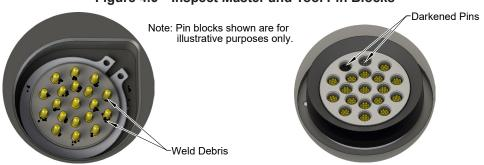
Tool Module Pin Block
