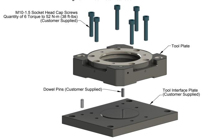
Figure 2.2—Tool Plate Installation
