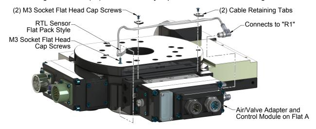
Figure 5.7—RTL (R1) Sensor Assembly Replacement with Master Cleat
