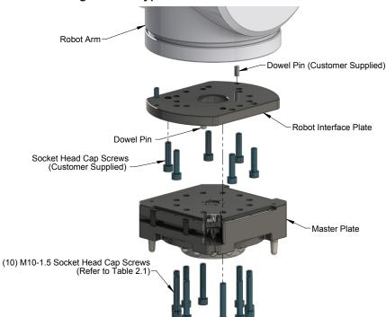
Figure 2.1—Typical Master Plate Installation
