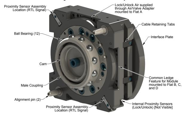
Figure 1.1—Master Plate Assembly
