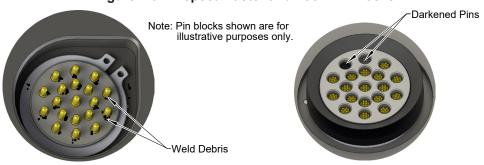
Tool Module Pin Block
