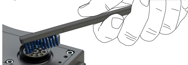
Figure 4.10—Clean Pin Blocks with a Nylon Brush
