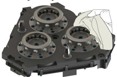
5. Use a clean rag to thoroughly remove any lubricant and debris from the inner surface of the male coupling and cam.
