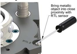
Figure 5.21—RTL (R1 and R2) Sensor Cable LEDs
