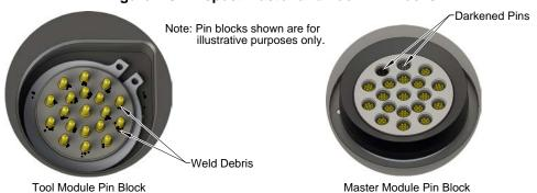
5. If debris or darkened pins are present, use a vacuum to remove the debris, and clean using a nylon brush (ATI part number 3690-000064-60).
