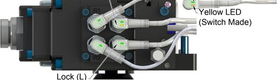
21. Confirm the operation of the Lock sensor by locking the Tool Changer and then checking to see if the lock sensor cable LED is on.
