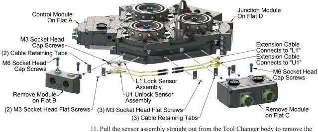
11. Pull the sensor assembly straight out from the Tool Changer body to remove the Lock and/or Unlock sensor assembly from the cable channel of the Tool Changer body. There is an O-ring around the cylinder barrel, ensure O-ring came off with old sensor before continuing. Discard the removed sensor assembly.
