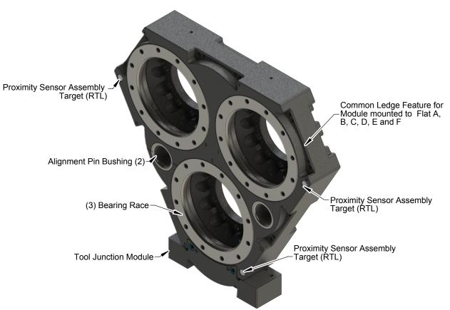
Figure 1.2—Tool Plate Assembly
