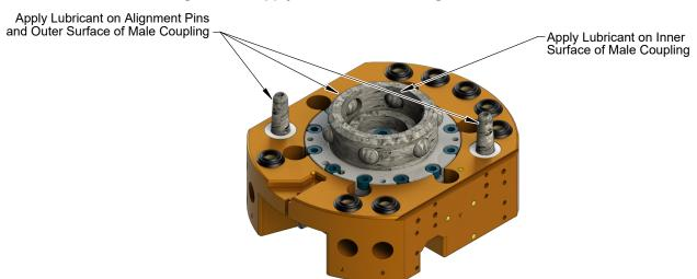
8. Use a clean rag to thoroughly remove any lubricant and debris from the Tool plate bearing race and bushings.
