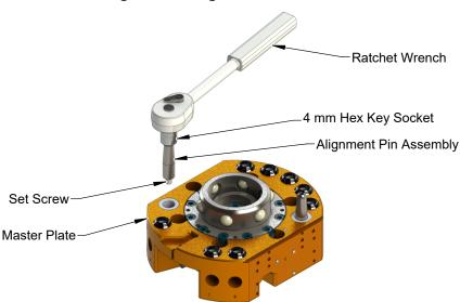
Figure 5.2—Alignment Pin Removal
