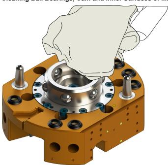
6. Check each ball bearing to make sure it moves freely in the male coupling. Additional cleaning may be necessary to free up any ball bearings that are sticking in place.
