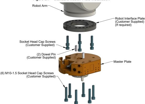
Figure 2.1— Standard Master Plate Installation
