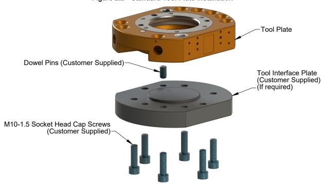
Figure 2.2—Standard Tool Plate Installation
