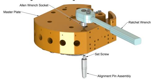
Figure 5.3—Remove Alignment Pin From Back Side
