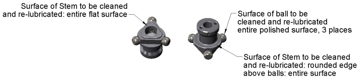
Figure 5.3—Cleaning and Re-lubricating the Stem
