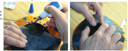
Apply Loctite to this Side of Stem6. Place the upper retainer onto the stem. Thread the flat head socket head cap screws into the tapped holes in the stem. Tighten screws to 96 in-oz (0.68 Nm).
