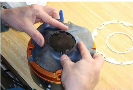
5. Apply the Loctite BlackMax 380 Instant Adhesive to the other side of the stem and then affix the boot to the other side of the stem.
