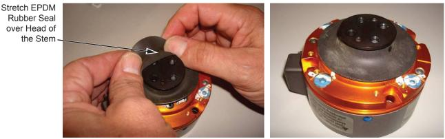
3. Place the weld splatter shield over the top of the stem and EDPM rubber seal and push down to the cover. Line up the slots in the weld splatter shield with the screw holes in the cover.
