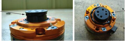
Apply a bead of Form-A-Gasket to Surface
