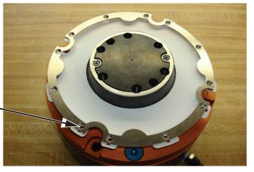
5. Thread the flat head socket head cap screws into the tapped holes in the cover plate and progressively thread them down. Tighten these screws to 32 in-oz (0.23 Nm).
