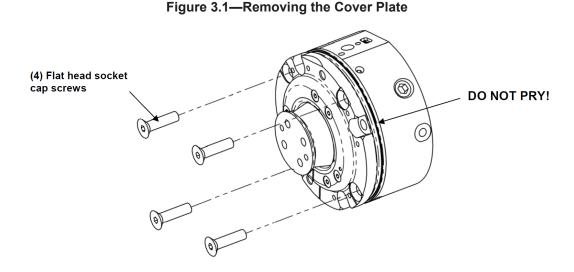
2. Remove the cover plate by carefully pulling it straight up and off of the body. This may be difficult due to the close fit of the dowel pins used to align the parts and the sealer used between the cover and body. It may be necessary to tap the cover with a rubber or plastic mallet.
