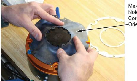
Figure 3.9—Determining Correct Orientation of Boot
