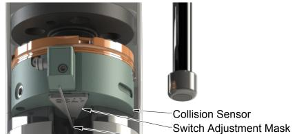
Figure 2.18—Locating of Adjusting Screw with Mask
