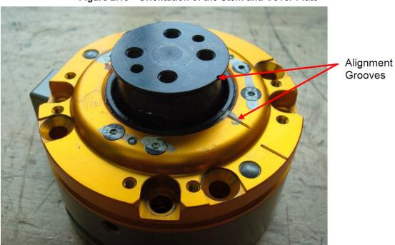
Figure 2.15—Orientation of the Stem and Cover Plate
