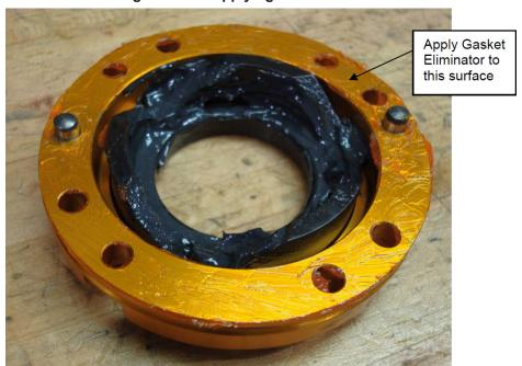
Figure 2.14—Applying Gasket Eliminator
