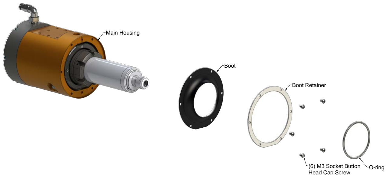
Figure 6.4—Spindle Boot Replacement
