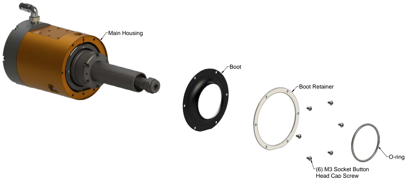
Figure 6.5—Spindle Boot Replacement
