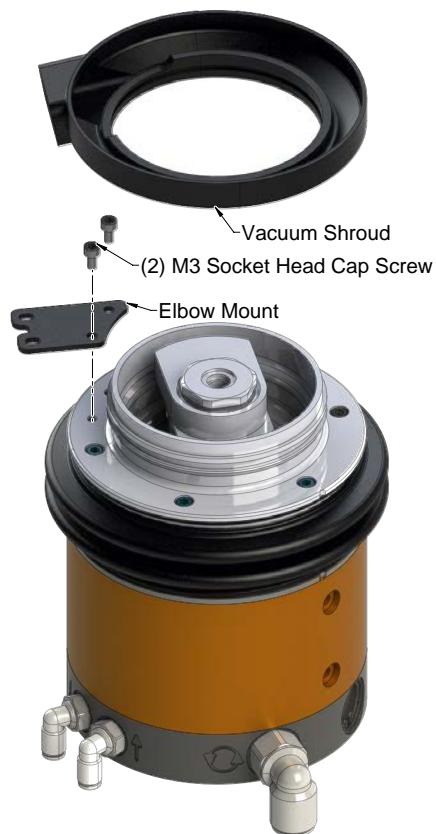
Figure 6.4—Remove Vacuum Shroud
