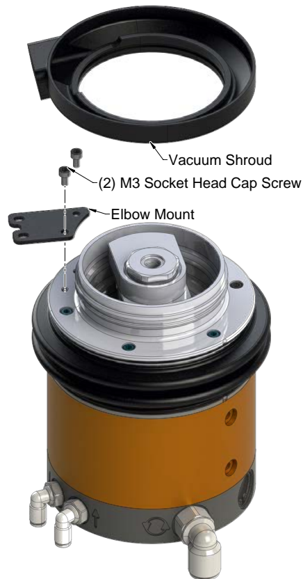
Figure 6.5—Install Vacuum Shroud
