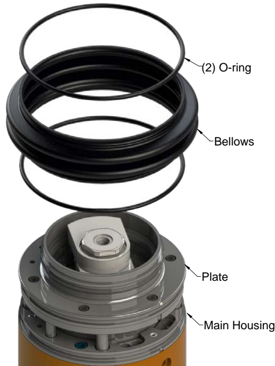
Figure 6.8—Dust Bellows Replacement
