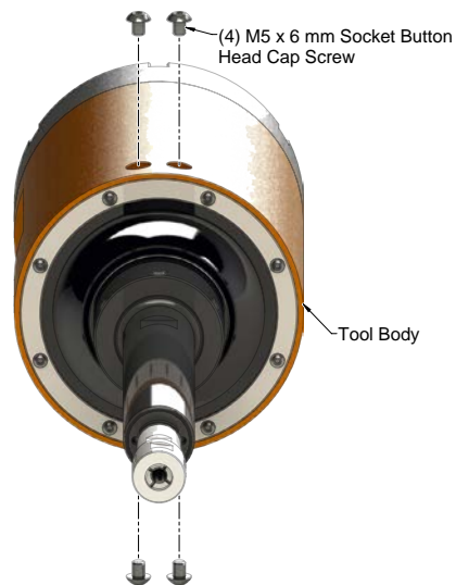
Figure 4.3—Remove M5 Button Head Socket Cap Screws
