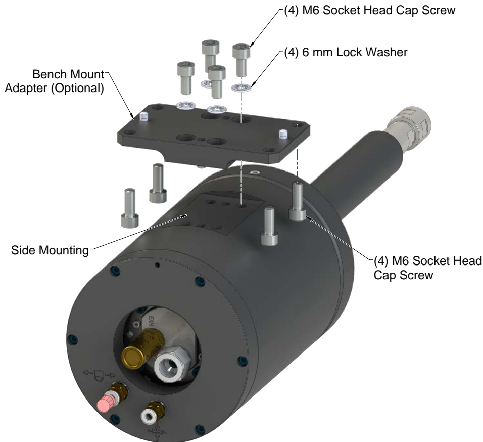
Figure 3.1—Side Mounting Installation
