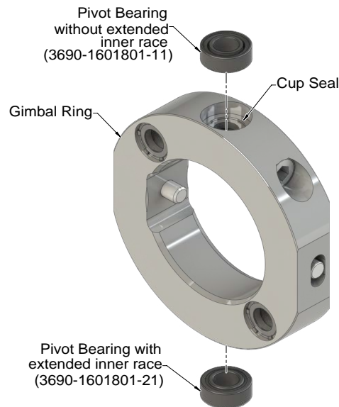
Figure 6.10—Gimbal Pivot Bearing Replacement
