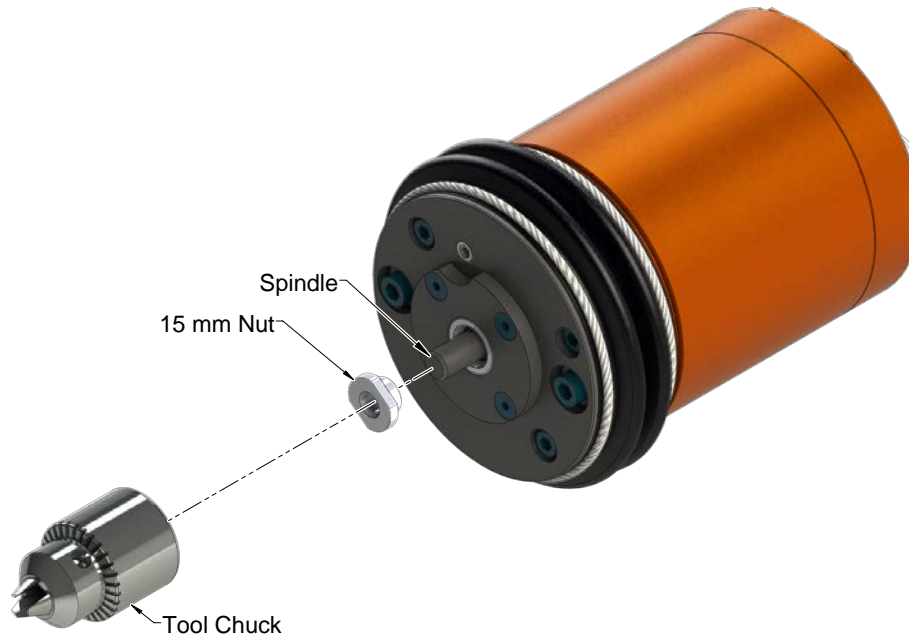
Figure 6.7—Installing the Chuck
