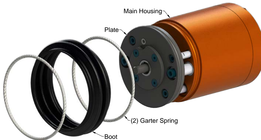
Figure 6.1—Flexible Boot Replacement
