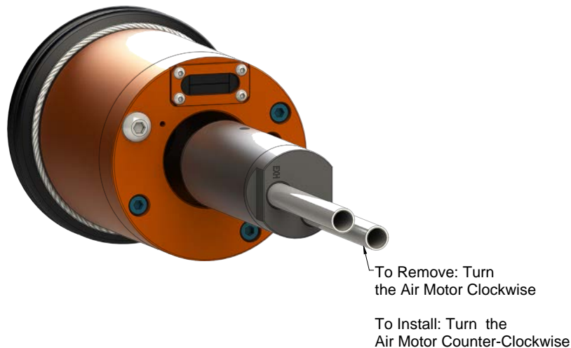
Figure 6.6—Replacing the Air Motor
