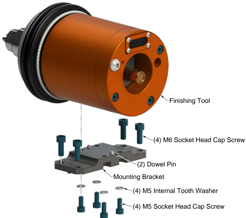
Figure 3.1—Side Mounting
