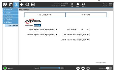
Figure 4.11—Enable Lock and Unlock Sensing
