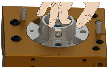
7. Apply a liberal coating of lubricant to the ball bearings, the male coupling (inside and out), and the alignment pins.
