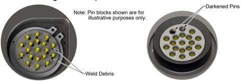
Tool Module Pin Block
