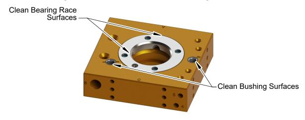
8. Use a clean rag to thoroughly remove any lubricant and debris from the Tool plate bearing race and bushings.
