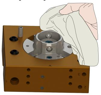
5. Use a clean rag to thoroughly remove any lubricant and debris from the inner surface of the male coupling and cam.
