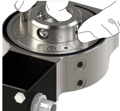
Figure 5.3—Check Ball Bearing Movement
