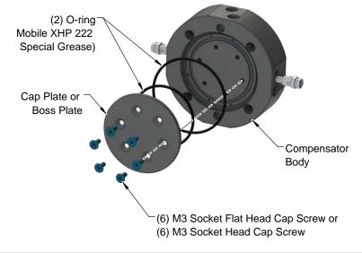
**NOTICE:** Use MobilGrease XHP222 Special grease to lubricate the locking mechanism and O-rings. Note: MobilGrease XHP222 Special is a NLGI #2 lithium complex grease with molybdenum disulfide.
