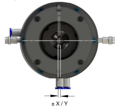
Figure 2.3—Lateral Compliance in the X and Y Axis
