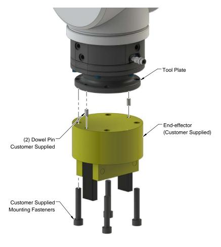
Figure 3.2—Installing the End-effector to the Compensator
