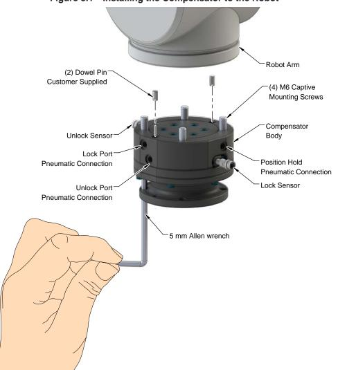
Figure 3.1—Installing the Compensator to the Robot
