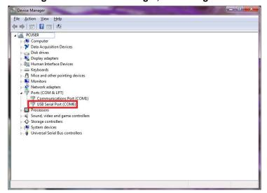
Figure 3.2—Device Manager, Port Assignment
