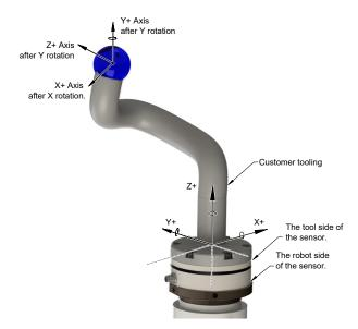
Figure 4.3—Tool Transformation: Rotation About the Y-Axis
