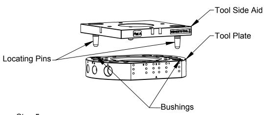
Step 5: Move the Master Plate Assembly slowly downward until the Master and Tool Side Aids are approximately 1mm apart.
