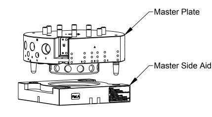
Step 6: Adjust the position of the robot to correct for any lateral misalignment. Use the Alignment Marks to align the Tool Side and Master Side Aids.
