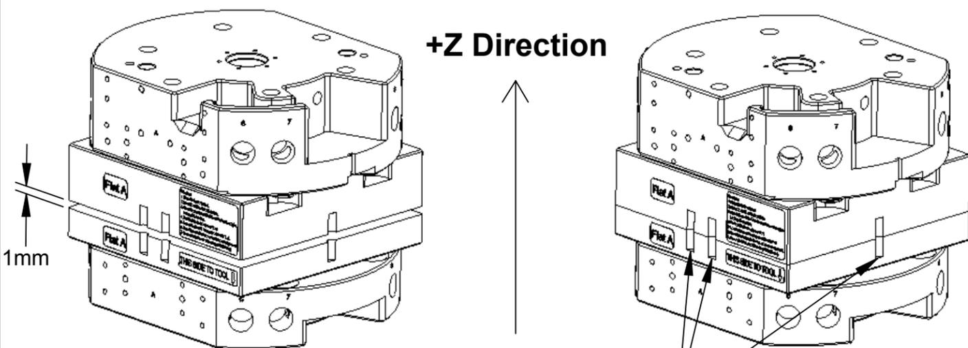
Ensure that the Tool Side and Master Side Alignment Marks are precisely aligned.
