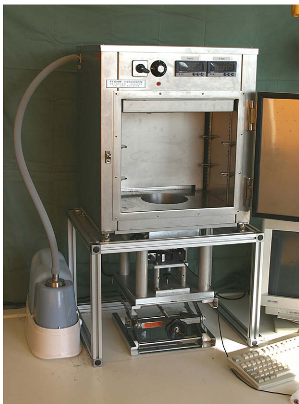
Fig 3. The entire measuring device is placed under a drying chamber, which has a hole in its bottom.
