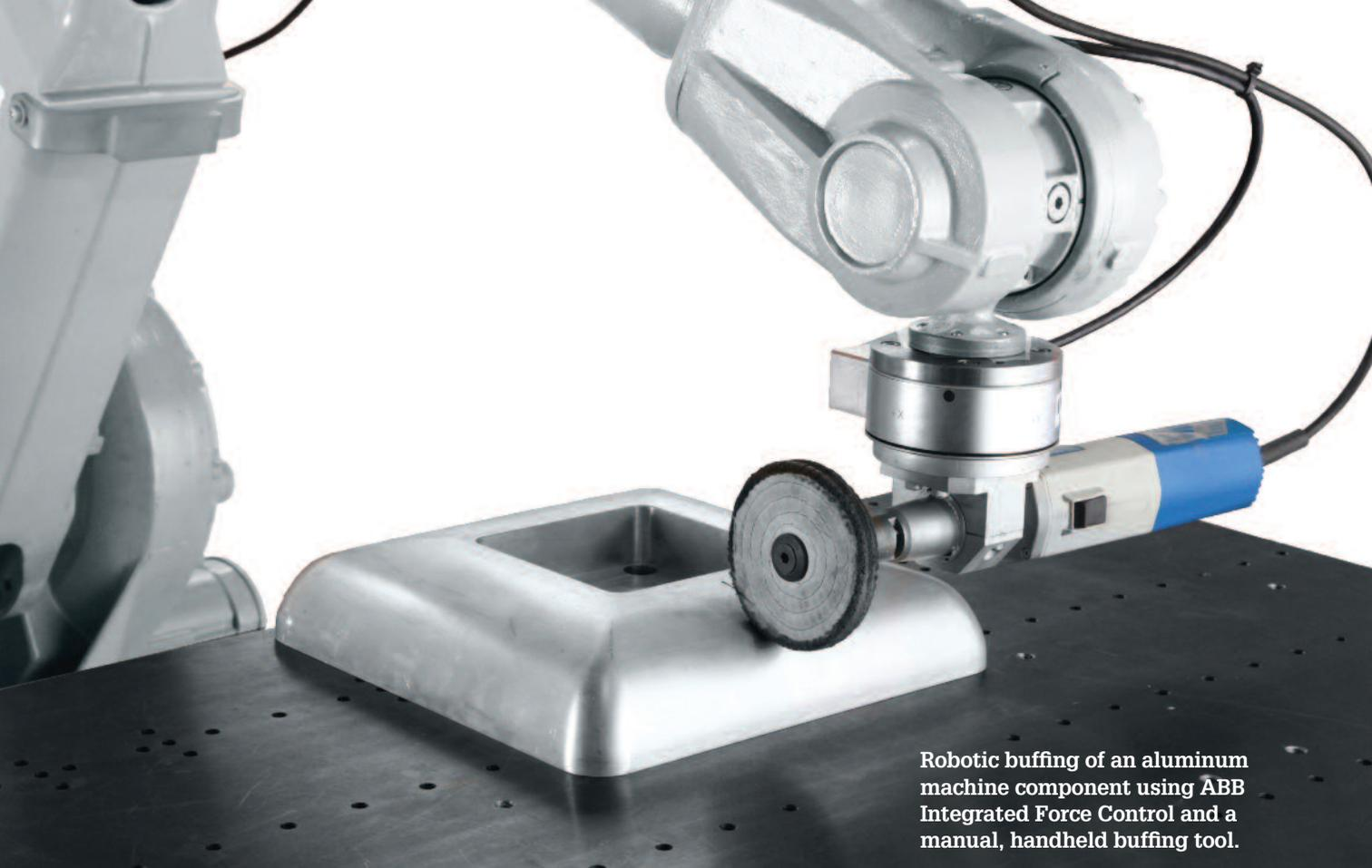
**Robotic buffing of an aluminum machine component using ABB Integrated Force Control and a manual, handheld buffing tool.**
