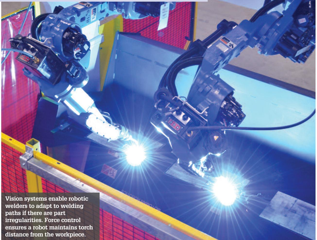
Vision systems enable robotic welders to adapt to welding paths if there are part irregularities. Force control ensures a robot maintains torch distance from the workpiece.
