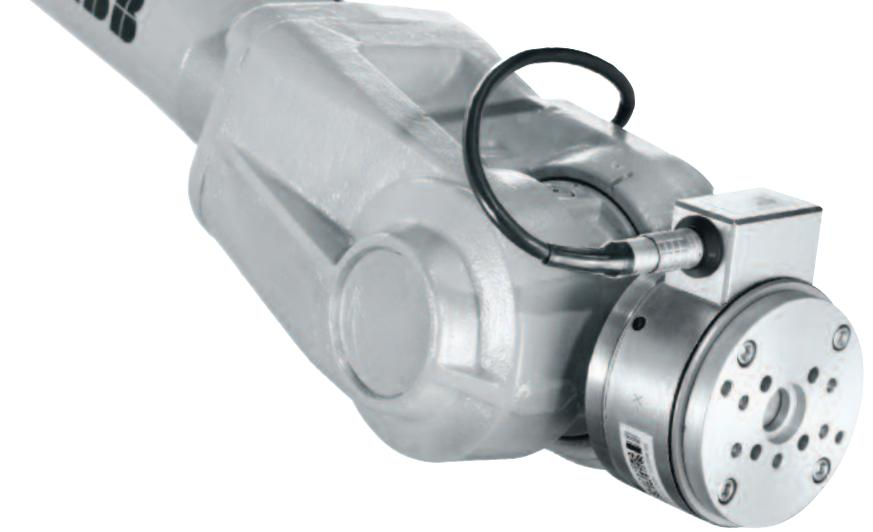
**Force control sensors, like the one attached to the end of this robot, precisely govern how much force an end effector applies during a job.**
