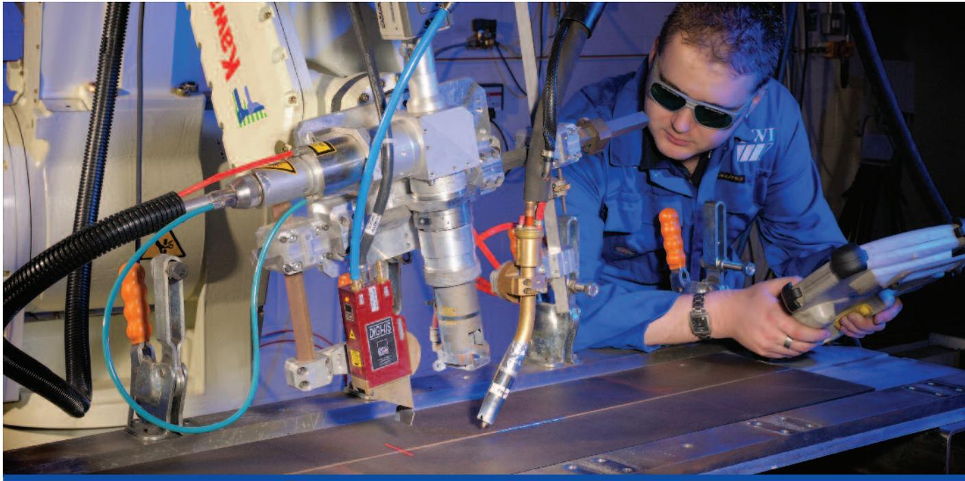
**Servo-Robot's adaptive vision systems give this hybrid laser-arc welder the flexibility to compensate for material warpage, should the material shift out of place. The robot keeps welding, without downtime.** Photo: TWI Ltd.
