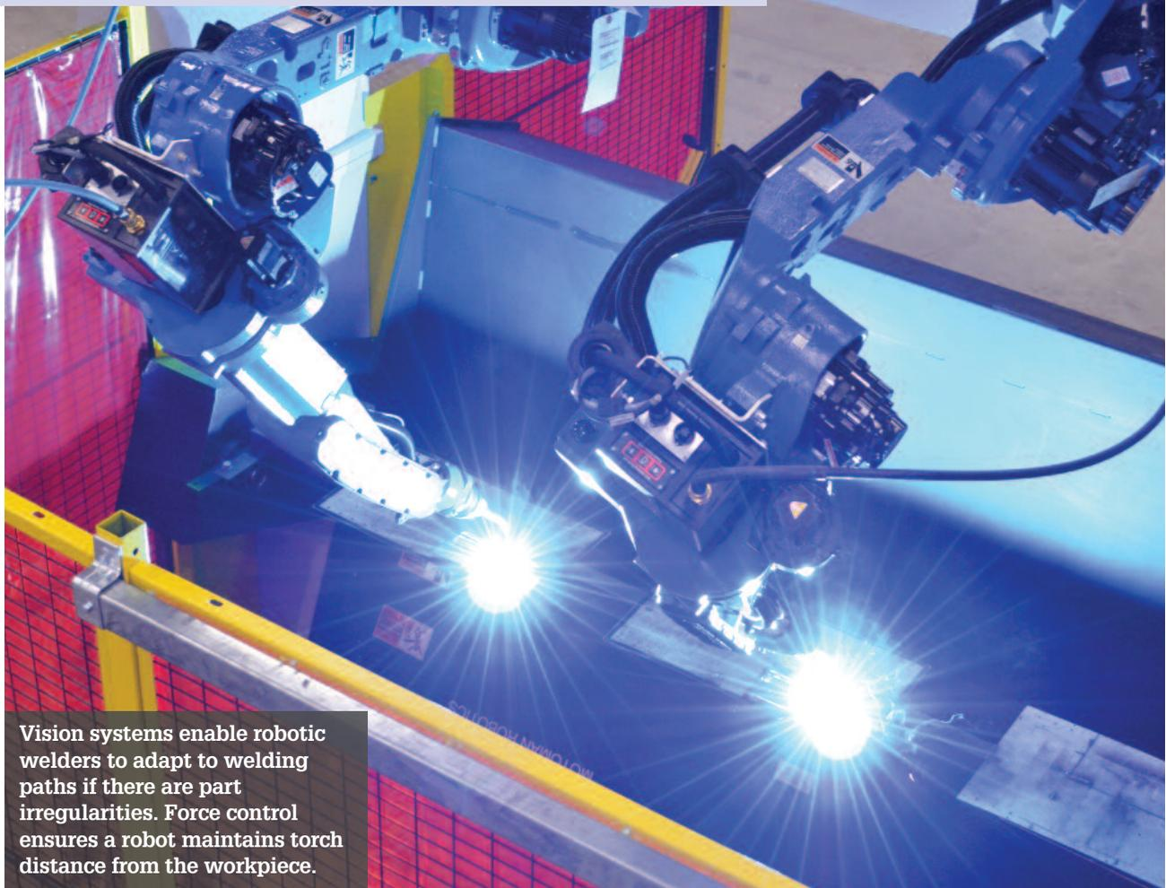
Vision systems enable robotic welders to adapt to welding paths if there are part irregularities. Force control ensures a robot maintains torch distance from the workpiece.
