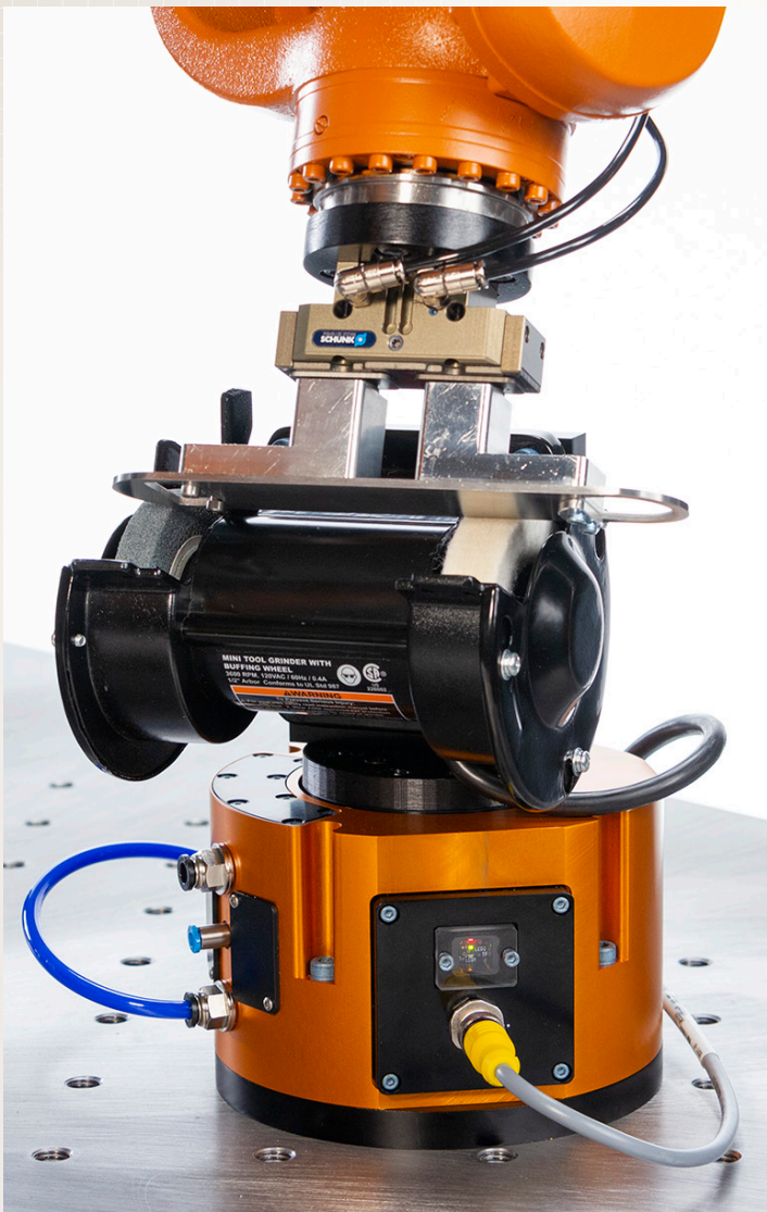
The PCFC can be bench mounted for optimizing part-to-process operations.
