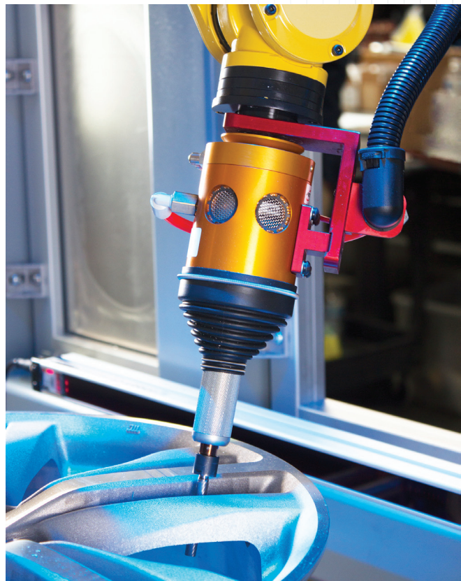
iA-Robotics pioneers a robotic system for high-precision, automotive wheel deburring.
