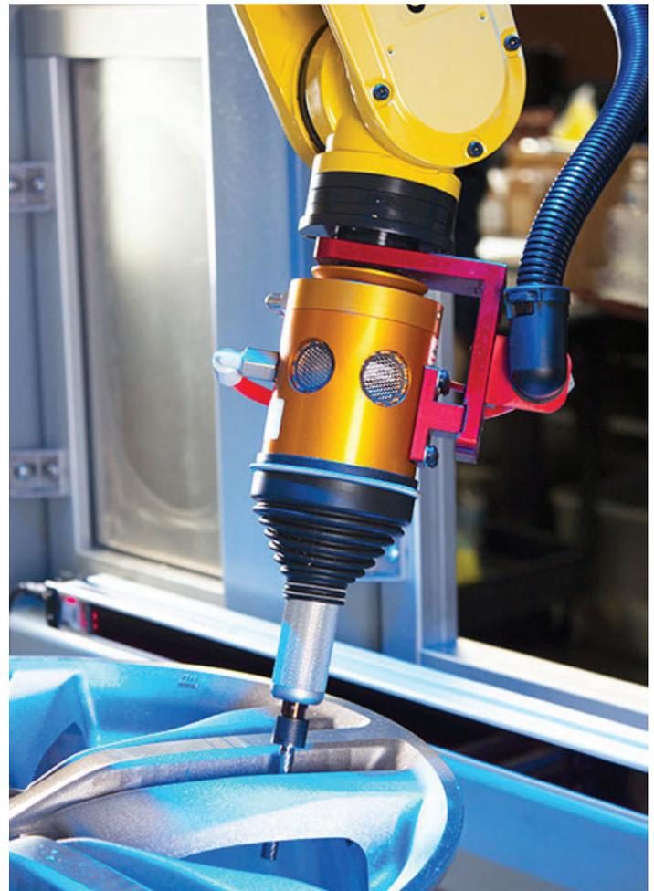
ATI’s deburring tool in action with iA-Robotics
