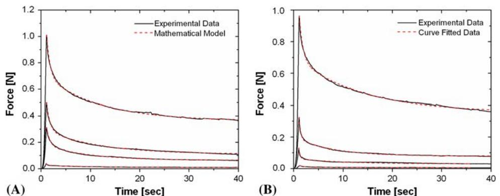
**Fig. 9** Model for elastic response of liver (A, B) and stomach (C, D): (A, C) Tangential elastic stiffness–force curve (B, D) experimental data and mathematical model for elastic response
