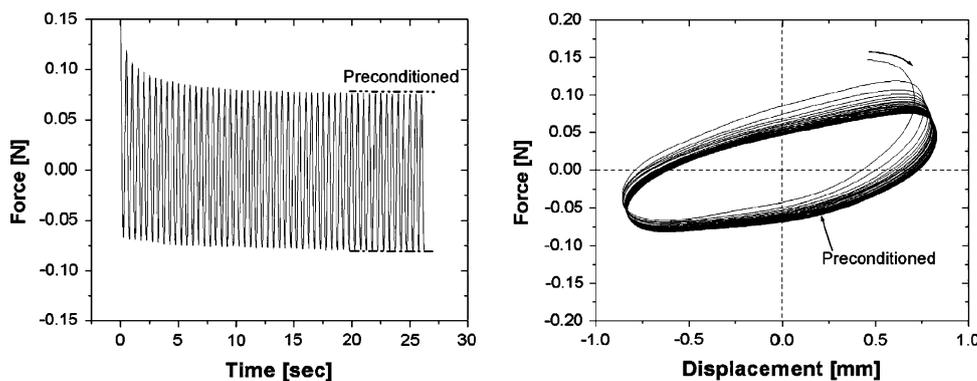
with various amplitudes (0.5–1 mm) superimposed on a pre-indentation of 4 mm to ensure that the indenter stayed in contact with the organ over the entire application of the load.
