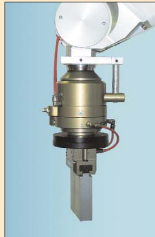
After Tooling Rotation. Note that lines to robot stay straight and lines to tool stay with the tool.
